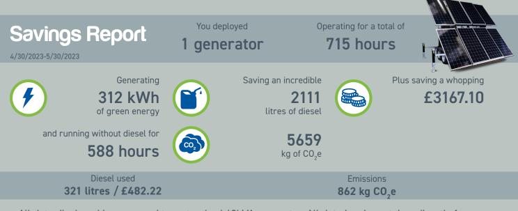
All data displayed is compared to a standard 40kVA generator. All data has been taken directly from the Prolectric Power Portal.
